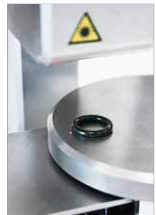
Laser centering and thickness measurement
