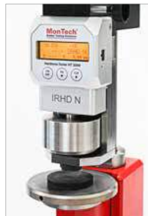
IRHD Normal measurement on parts
