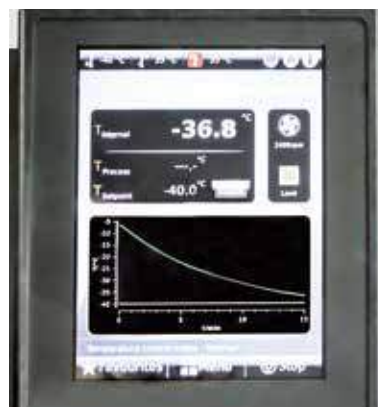
Sample temperature recording by optional immersion probe
