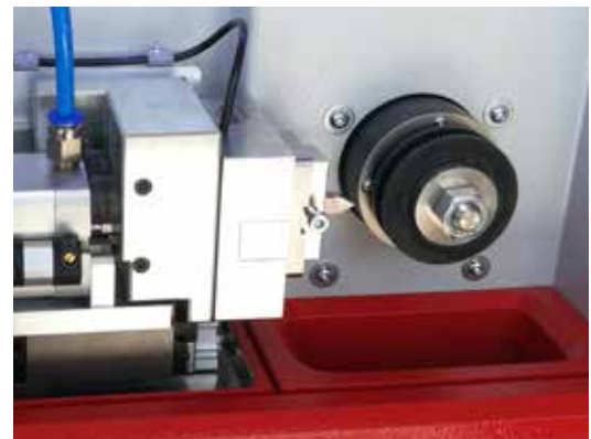
Closed loop controlled cut and chip actuator with multi-axial force sensor
