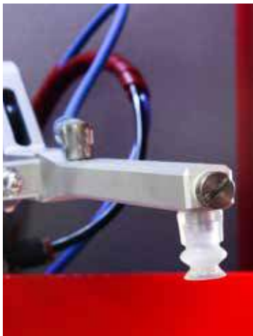
High volume vacuum handling of samples guarantee proper sample handling and placement.
