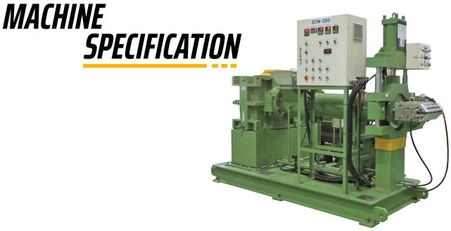
**Overview** It is a machine consisting of a spiral worm which rotates in the barrel. As for the worm and barrel threads, the temperature can be set as needed. The rotation of the worm screw will cause the compound to continuously enter the barrel and create pressure for the compound to flow through the die in the front to form a shape.
