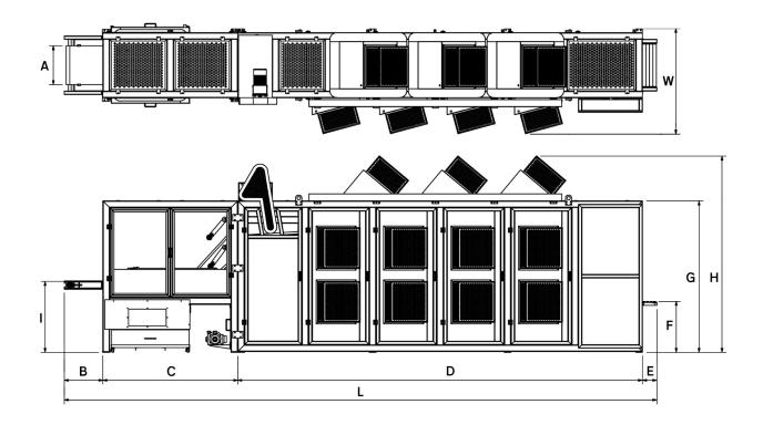
**Overview** The most common type of batch off machine is the Horizontal type. It is a rubber dryer machine that is commonly being used by most of our clients. The horizontal batch off is consisted of 5 - 7 layers of belt laying horizontally so that the rubber sheet can lay on the belt. It comes with a ventilation system by fans along the conveyors.
