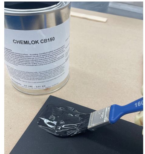
Figure 4. Apply to Prepared Rubber
