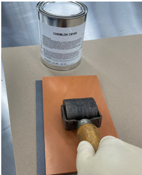
Figure 6. Mate and Stitch Rubber to Metal
