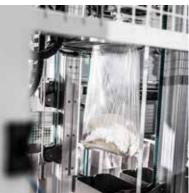
allows precise and safe automatic dosing operations of the products, required for the preparation of powder dyes and chemicals in automatic thermoformed bags, starting from tubular films (EVA, LDPE, ...)
