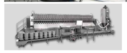
is a fully automatic weighing system for powder ingredients, granting constant quality and thorough control over color masterbatch preparations.
