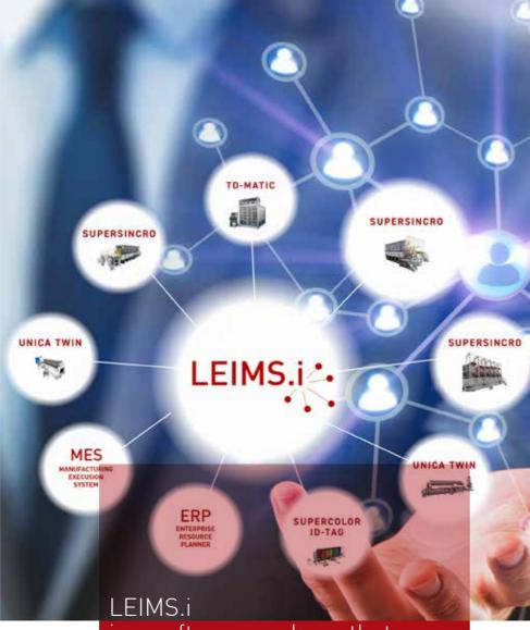
is a software package that manages a whole Lawer plant. This tool allows connecting management and program systems, to import production orders and assign them to the machines of the plant.
