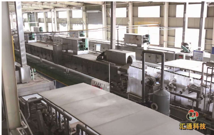
The base has established high-alkali glass block production line used for glass fiber cotton, with an annual output of 30,000 tons.
