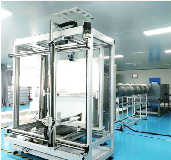
↑ Vertical EN-1822 Test System
