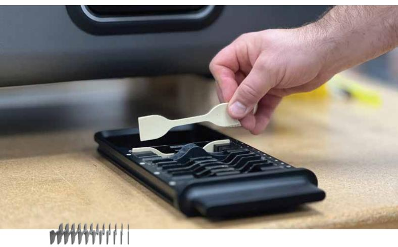
Load up to 12 tensile and tear samples per tray for faster, more efficient testing.
