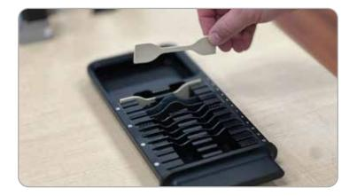
Simply load up to 12 tensile samples, with your choice of mixed compounds and different materials.
