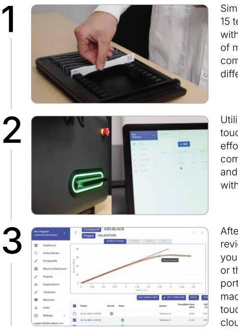
Simply load up to 15 tensile samples, with your choice of mixed compounds and different materials.
